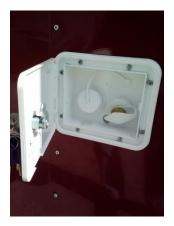
and fill your fresh water tank from here, from either a food grade hose or other water source, depending on what you require. There is also a female hose bib fitting behind the door. If fresh water is available to you to run your concession, you can simply connect a food grade hose to the water supply and connect the hose to this fitting. Turn the water on, and your concession sinks will operate from the water pressure created from the hose and the water pump will not need to run at all.
