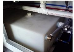
greater in capacity. The fresh water tank is typically located under or near your sinks inside the trailer. Maintenance will include periodically checking to make sure the threaded fitting are snug and not leaking. Also check to make sure there are no kinks in the small clear vent hose.
